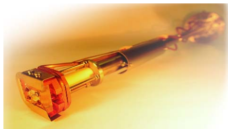
Fig. 2 Laser heated UHV and ambient pressure XPS stage
